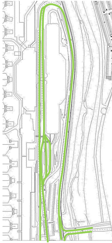
Figure 4-3: Terminal A – High Scenario Roadway LOS
