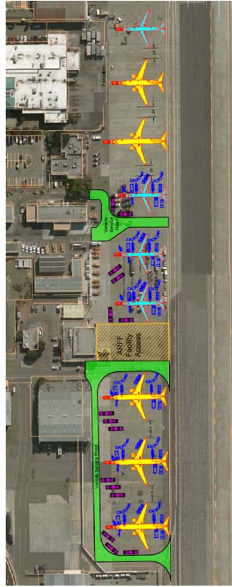
Figures 2-5.1: South Apron RON Parking
